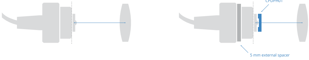
Add a 5 mm external spacer and add CPDPH01
